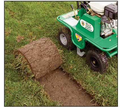
Cuts Turf Clearly & Evenly 12" cutting width and up to 1.38" deep.
