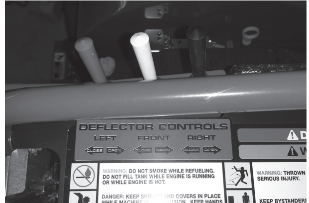
Deflector Control Switches
